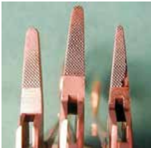
Signs of wear of the tungsten carbide insert necessitating repair.
